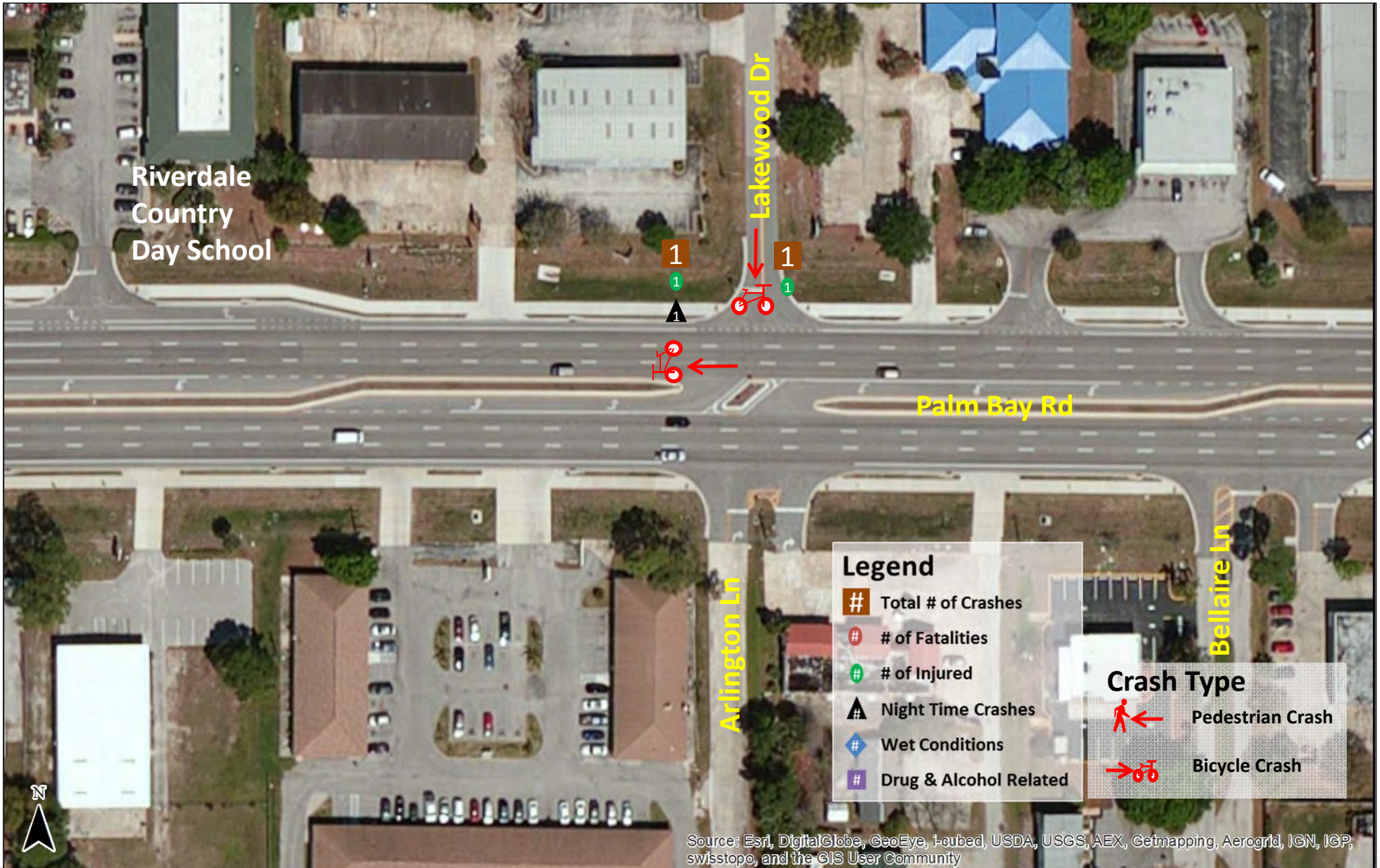
Palm Bay Road Ped/Bike Field Review Collision Diagram (2009 – 2014) Lakewood Drive to Bellaire Lane
