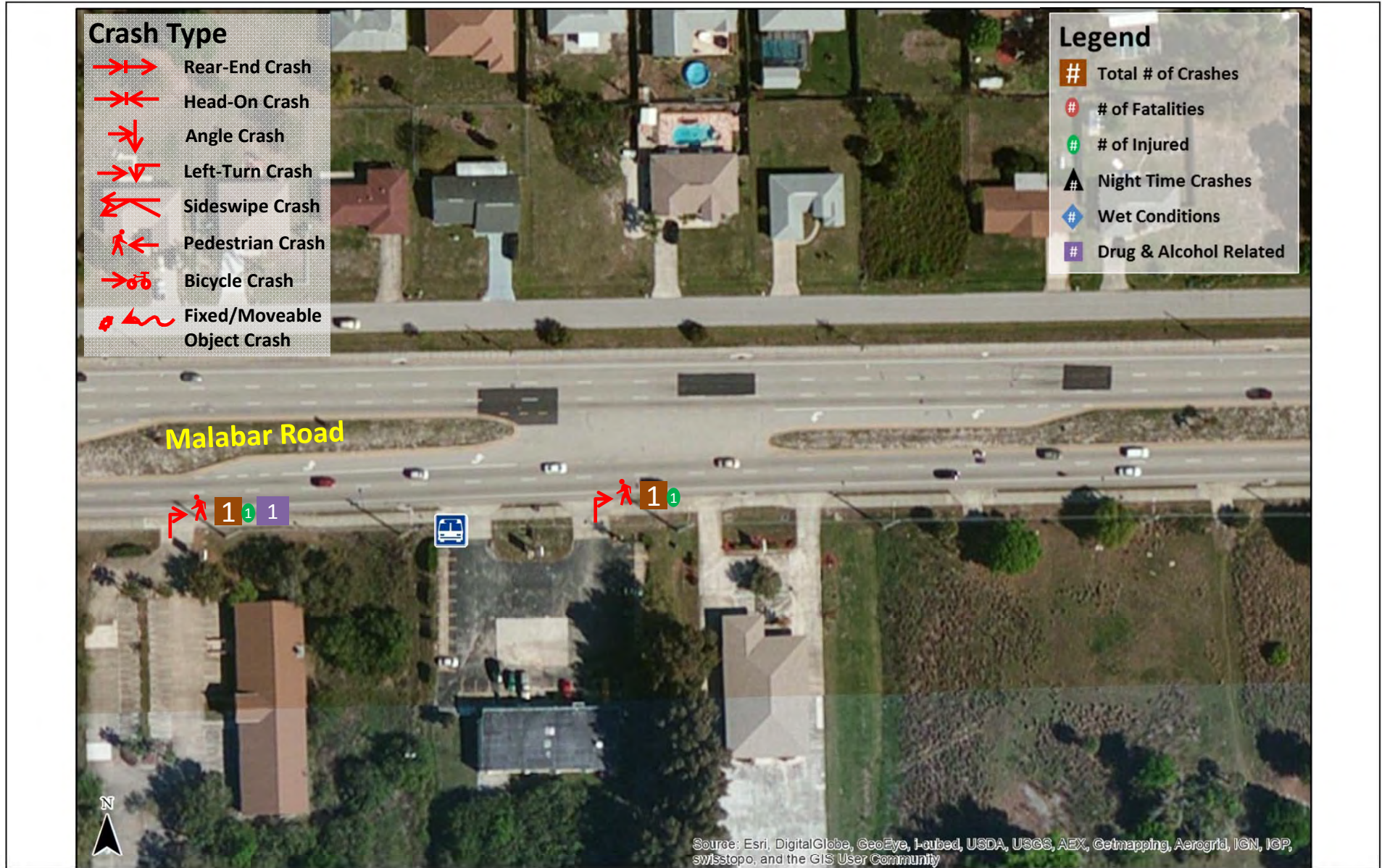
Malabar Rd. (Jupiter Blvd. to Minton Rd./Emerson Dr. to San Filippo Dr.) RSA Collision Diagram (2009 – 2014) Segment 2 Emerson Dr. to Corporate Cir.
