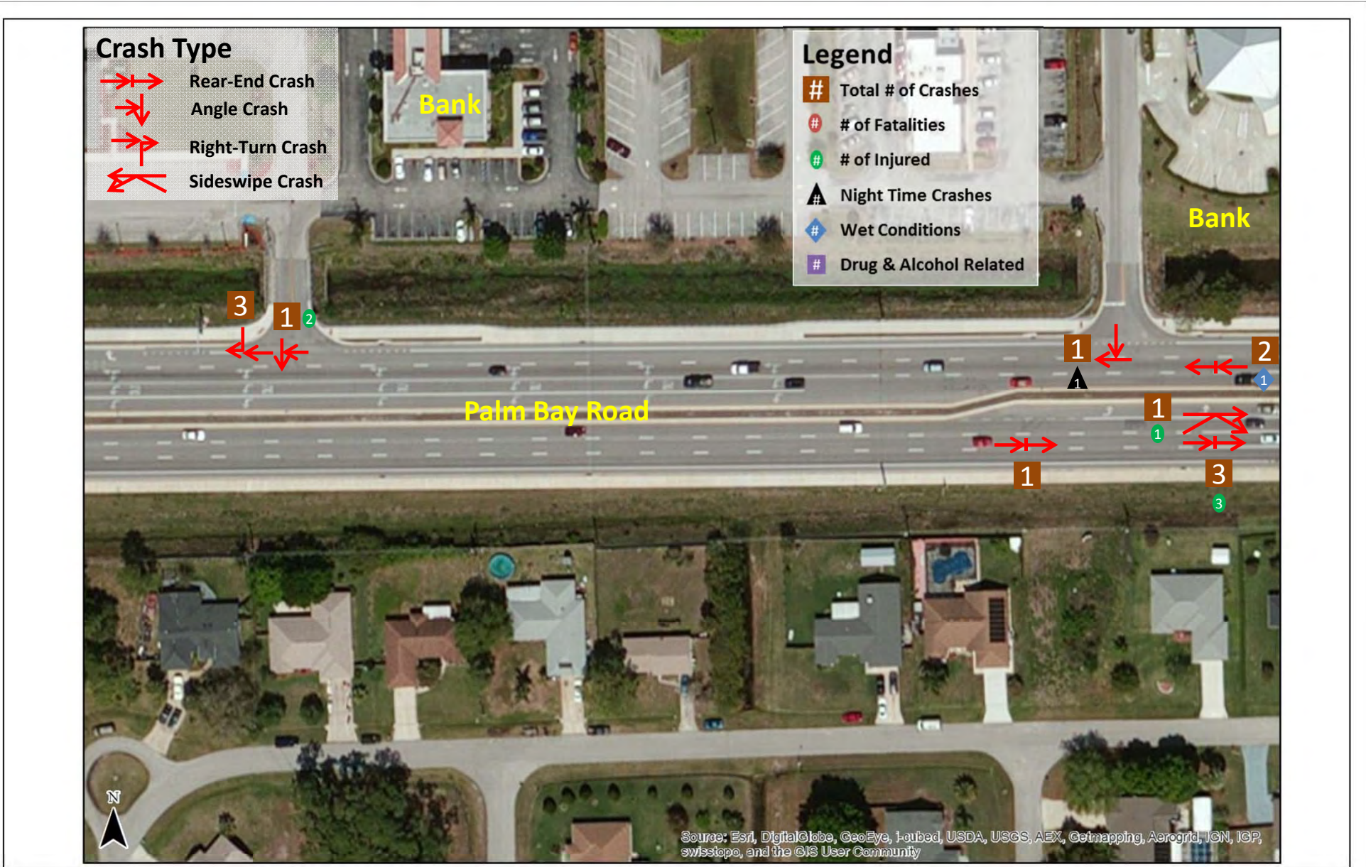
Emerson Drive (Jupiter Boulevard to Culver Drive) RSA Collision Diagram (2009 – 2014) Intersection 4/5: Palm Bay between Minton and Athens
