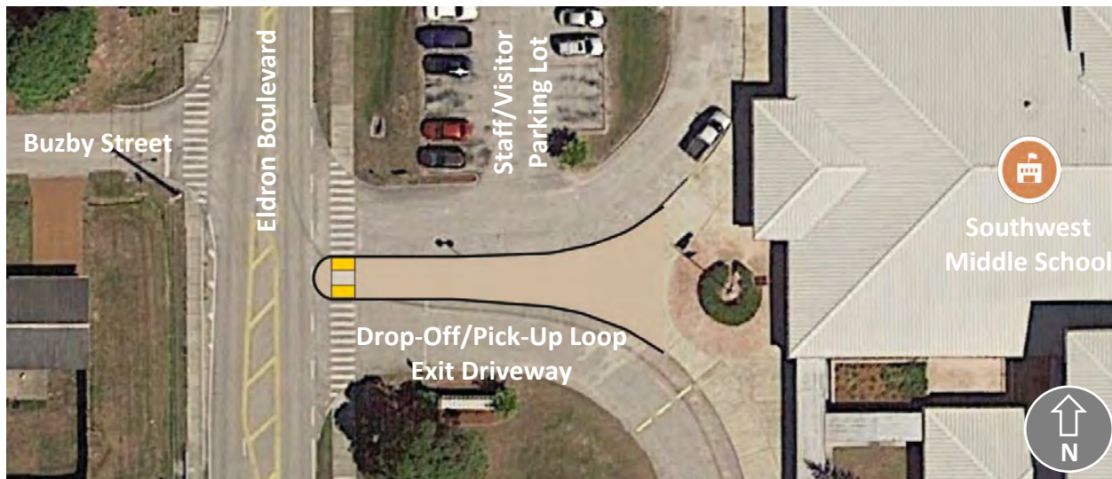
Extended Concrete Separator in Blue Between Drop-Off/Pick-Up Loop Exit Driveway and Staff/Visitor Parking Lot Entrance Driveway
