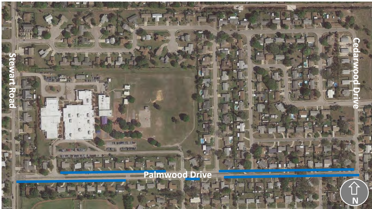
Sidewalk Gaps on Palmwood Drive in Blue
