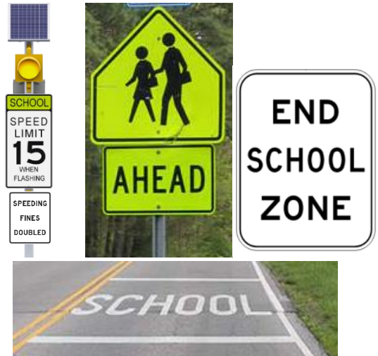
Proposed Flashing Beacon, Marked School Crossing, End School Zone, and School Pavement Markings
