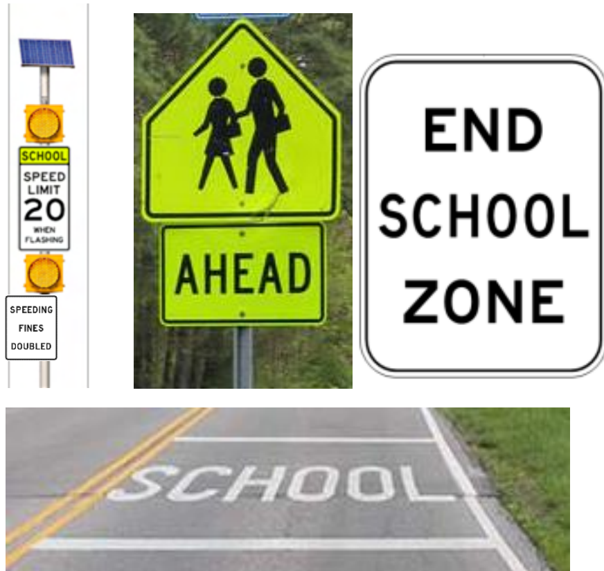
Example of Flashing Beacon, Marked School Crossing, End School Zone, and School Pavement Markings
