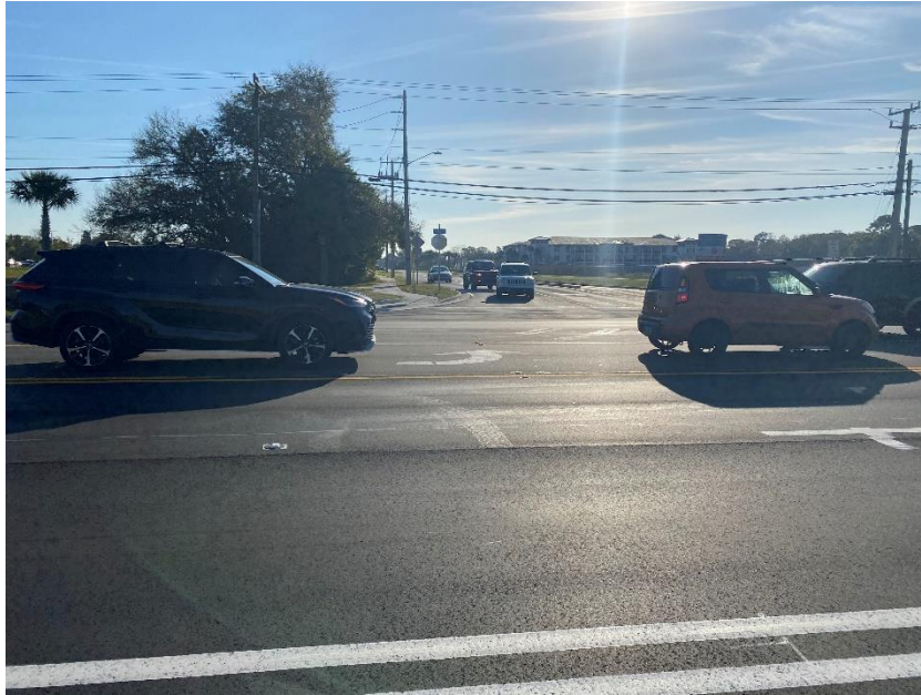
Figure 4: Left-Turning Vehicles Staging in Center Turn Lane on Fiske Boulevard
